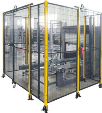
Fig. 11 Perimetral safety protections CAR
