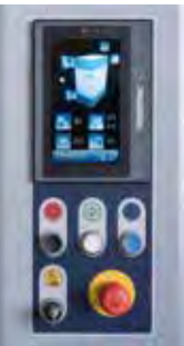
Pannello touch screen con tecnologia "Multilevel Control". Touch screen control panel with "Multilevel Control" technology.
